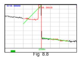
The LSA area and cursor are set too late. The left green LSA indicator line is not over laying the back scatter of the trace properly.
