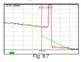
The LSA area and cursor are set too early. The right green LSA indicator line is not over laying the back scatter of the trace properly.
