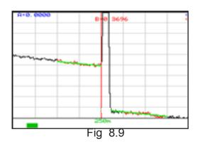
The LSA area and cursor are set properly. The green LSA indicator line is over laying the back scatter of the trace properly.
